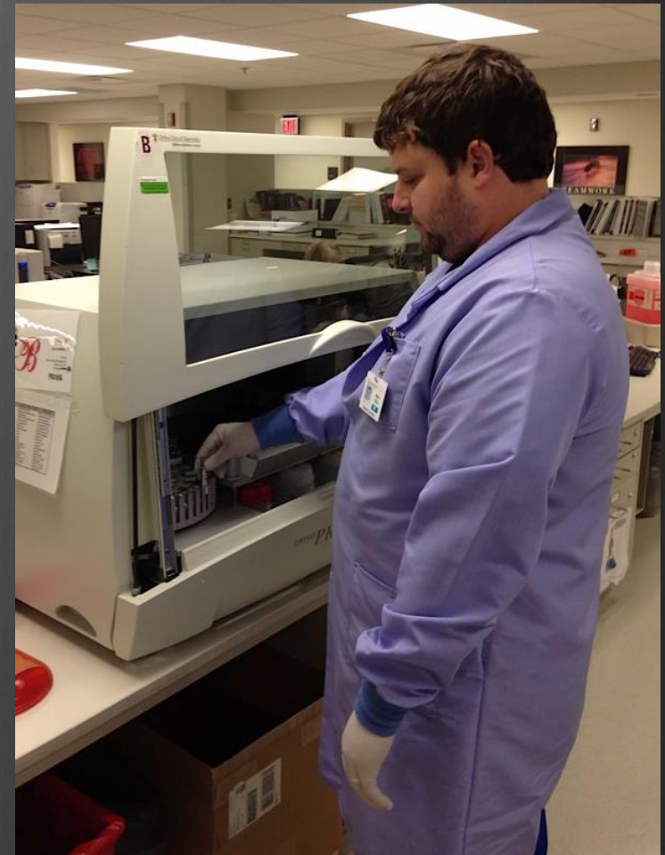
Marc, Class of 2010, loading a specimen onto the Ortho Provue™ automated instrument that performs patient ABO and Rh typing
